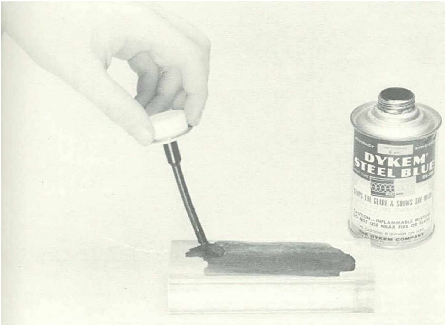
Fig. 6-1. Applying layout fluid preparatory to making the layout.
