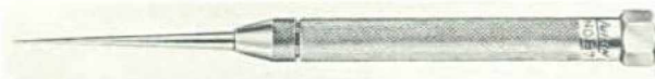
Fig. 6-2b. Pocket scriber. The point is reversed and stored in the handle when the tool is not being used.
