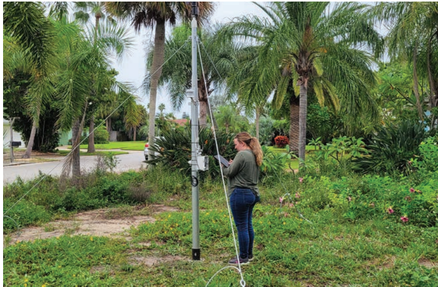
Graduate student Hadley Besing works on an R.M. Young anemometer in Satellite Beach, Florida. The device, which also included a HOBO temperature/humidity sensor package and additional pressure sensor, would later collect wind speed data from Hurricane Ian.
