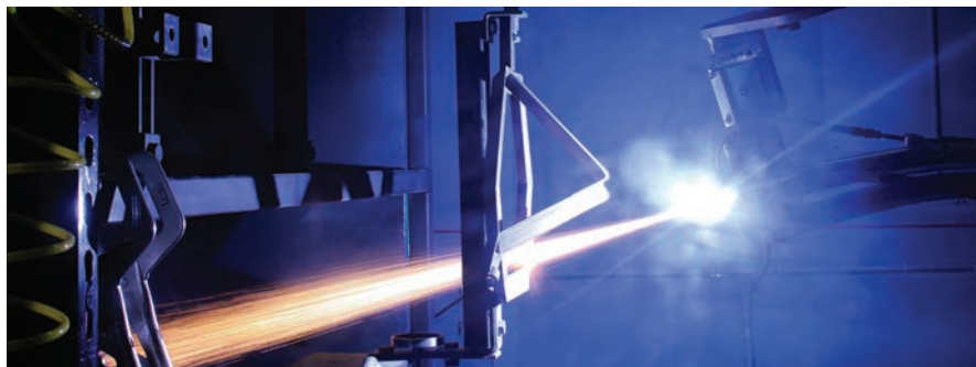
The Plasma Spray Thermal Lab at Florida Tech's Center for Advanced Coatings features a spray gun that melts ceramic powder onto test material at high speeds.
