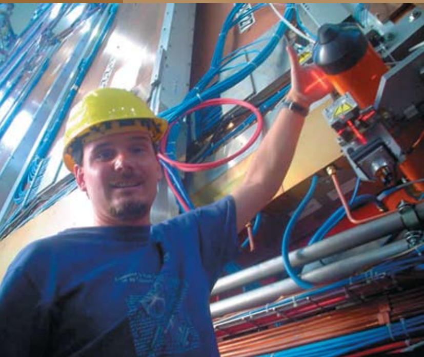
(left) Marcus Hohlmann checks the laser alignment system for the muon endcaps of the Compact Muon Solenoid detector at CERN.
