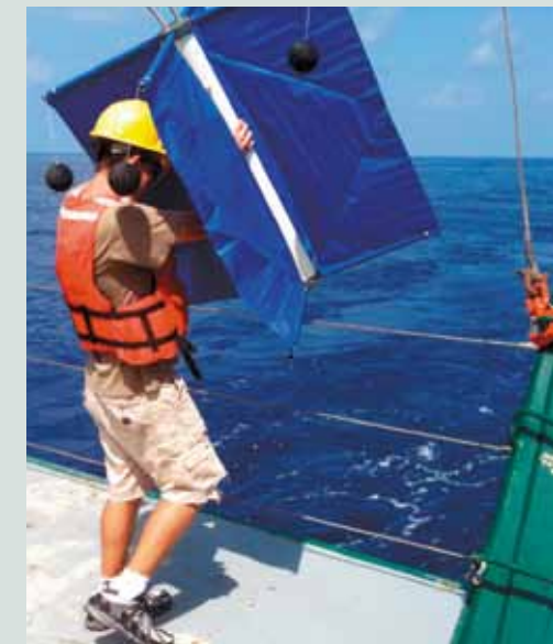
Student Skyler Goldman deploys a drifter buoy off the stern of the RV Weatherbird II.
