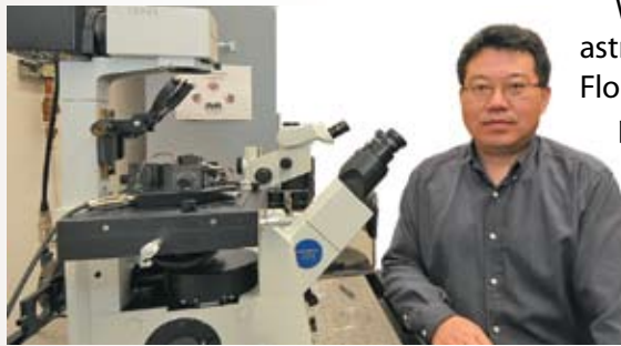
Dr. Shaohua Xu with the atomic force microscope that reveals how protein molecules stick together to form identical spherical particles.
