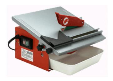
There's no substitute for a diamond saw when you have to make fine cuts—corners, curves, slivers—or cut stone or other hard material. The most distinguishing feature of a wet saw is a steady stream of water keeping the saw blade and the tile surface wet during operation. The water helps the blade grind through the tile without breaking it, keeps the blade cool to prevent overheating and significantly reduces the amount of dust that would otherwise be produced when cutting.
