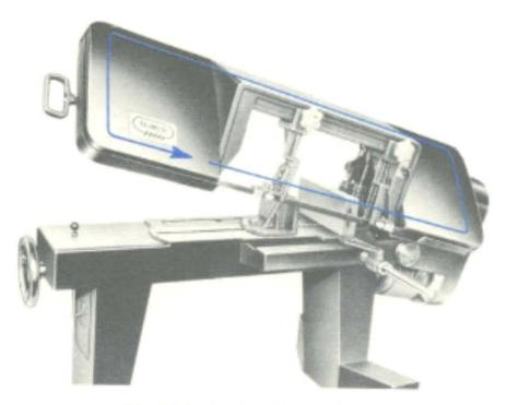
Fig. 35-2. Metal cutting band saw. (Kalamazoo Tank & Silo Co.)
