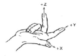
Machine tool axes are specified according to the "Right Hand System" of Cartesean coordinates. When the right hand is held as shown above, the thumb, forefinger and middle finger point in positive X, Y and Z axes respectively.
