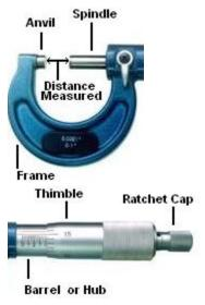
Note that the distance measured is the distance between the spindle and the anvil. The piece is inserted here, and the spindle length is adjusted so that the piece being measured just touches the anvil and the spindle.
