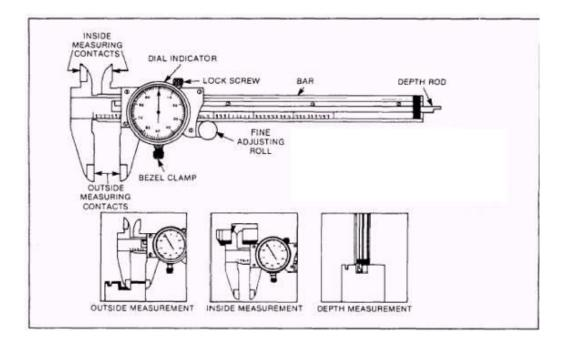
Calipers with a dial are much easier to read than the old dial-less slide vernier calipers. They eliminate eye strain. Always double check a caliper reading! Set the dial to zero in the closed position before measuring.
