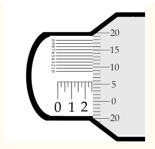
The above micrometer reads .250 on the Sleeve and .005 on the Thimble = 0.255. Now look for the vernier mark that lines up closest to any of the lines on the Thimble. In this case it is the vernier marked 8. The micrometer shown above reads 0.2558
