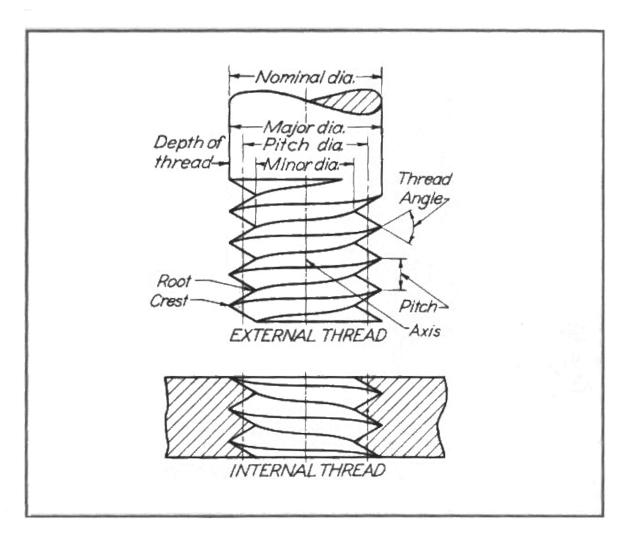
Major Diameter: the largest diameter of an external or internal thread
