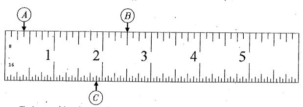
The bottom of the ruler is graduated in 1/16ths of an inch. Count the lines to take a reading but "count the lines odd"!
