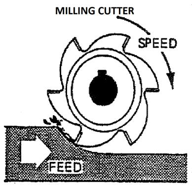
Consult the mill manual or wall chart for the speeds and feeds required for various materials. Cutting <u>Fluids</u> serve several purposes. They carry away the heat generated during the machining operation, act as a lubricant and prevent the chips from sticking or fusing to the cutter teeth, and flush away chips. The lubricating qualities also influence the quality of the finish of the machined surface.
