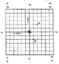
The quadrants formed when the X and Y axes cross allow any point to be accurately located from the X-Y zero point, or origin.
