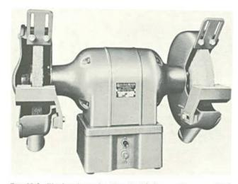
Fig. 33-2. The bench grinder. Eye shields have not been mounted.
