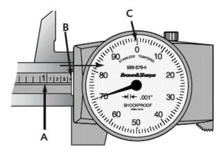
It might seem intimidating and complicated, in reality dial calipers are simple to read once you get the hang of it. You read it in the order A, B, C as the diagram above shows. If the hand on the dial is between two numbers you just need to estimate the reading. If you see the hand is exactly in the middle round up. That would make the reading showing on this dial caliper one inch, three hundred seventy thousandths.
