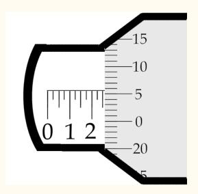
If this was a 0 - 1" micrometer it would read somewhere between 0.255" and 0.256". (.250 on the Sleeve, with more than .005, but less than .006 on the Thimble).
