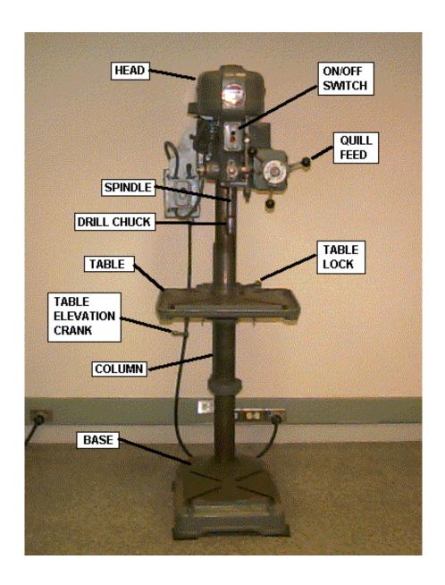
A powered vertical drilling machine in which the rotating bit is pressed to the work by a hand-lever. The work is secured to a table. The spindle speed is changed by selection of a pair of step-pulley grooves. Larger drill bits turn at slower speeds. Lubricant (cutting fluid) can be used to cool and improve cutting.
