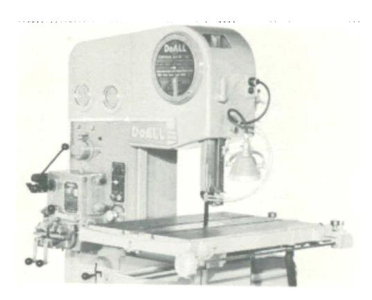
The Vertical Bandsaw has a moving bandsaw blade fixed in a vertical position while the material to be cut is fed into the blade by the operator's hands.
