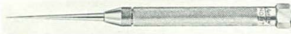
Fig. 6-2b. Pocket scriber. The point is reversed and stored in the handle when the tool is not being used.
