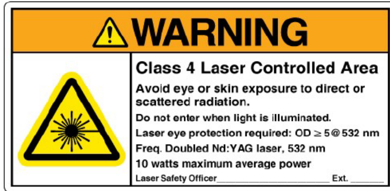
Figure 1. Sample ANSI Z535.2 Compliant Warning Sign (Class 3B and Class 4 LCAs)
