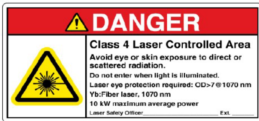
Figure 2. Sample ANSI Z535.2 Compliant Danger Sign (Class 4 LCAs)
