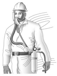
Tight-fitting Atmosphere-Supplying Respirator with an auxiliary escape bottle
