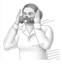
A user seal check is not a fit test. The user seal check is one step an employee must take before any fit testing is performed and before the employee uses the respirator in the workplace.
