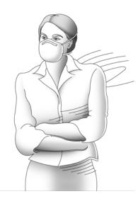
Half mask Filtering Facepiece Dust mask APF=10 Needs to be fit tested
