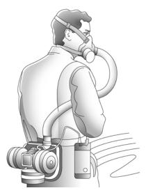
**Tight-Fitting Full Facepiece Powered Air-Purifying Respirator** (PAPR) APF= 1,000 *Needs to be fit tested*
