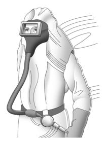
**Tight-fitting Abrasive Blasting Respirator Continuous flow** APF=25/1,000\* **SAR Full Facepiece** *Needs to be fit tested*\*
