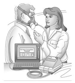
**Quantitative fit testing**. To conduct quantitative fit testing on an atmosphere-supplying respirator, you must temporarily or permanently install a sampling probe or adaptor inside the facepiece.
