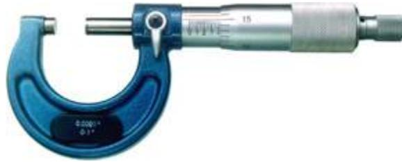
Pictured above is an "outside micrometer". This is a tool often used in manufacturing environments to make precision measurements of the outside dimensions of a piece. Let's take a look at some of the parts of this instrument:
