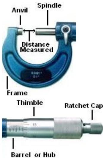
Note that the distance measured is the distance between the spindle and the anvil. The piece is inserted here, and the spindle length is adjusted so that the piece being measured just touches the anvil and the spindle.
