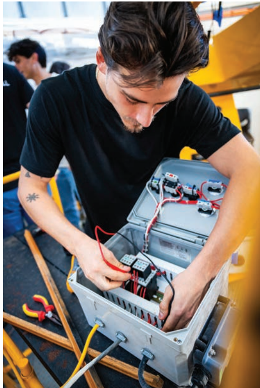
» Left: Student Lennox Krell uses a multimeter to test the electrical properties of one of the observatory's dome control boxes.
