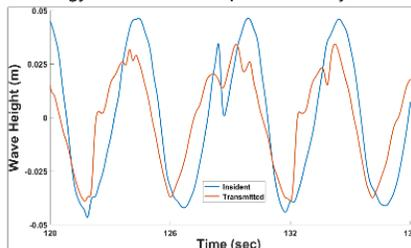
Figure 2: Oystercrete Wave Dampening Effects
