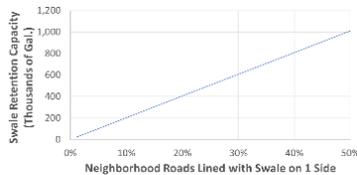
Figure 1: Gallons of Water Retained by Residential Swales
