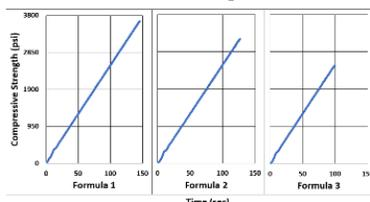
Figure 1: Compression Testing of Oystercrete Formulas
