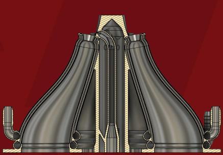
The metal 3D-printed radial aerospike engine represents a complex integration of advanced manufacturing, fluid dynamics, structural resilience, and data acquisition, culminating in a system designed for high-temperature, high-pressure static fire testing. The system-level components have been carefully developed to ensure a seamless and controlled testing environment at the Vaya Space facilities.
