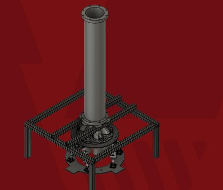
An altitude-simulating shroud compatible with the aerospike design will be placed around the nozzle. This shroud will create controlled, localized pressure drop, simulating ambient atmospheric conditions experienced at various altitudes during a rocket launch. Thrust and pressure data will be recorded to validate the performance of the shroud and to evaluate how the aerospike performs under reduced ambient pressure, assessing its altitude-compensating efficiency.
