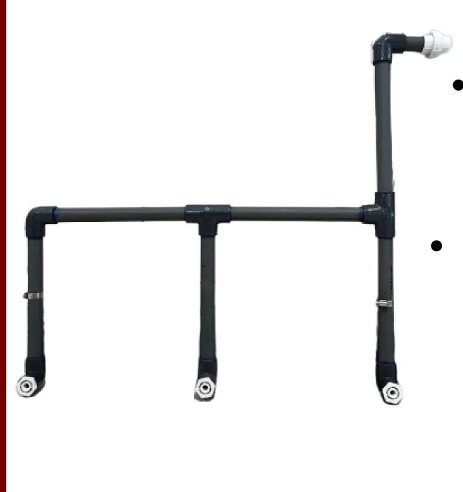
**Submerged Jets:** PVC piping system that is fitted inside of the waterjet tank. The jets homogenize and guide the fluid mixture towards an inlet pipe connected to the separation system.
