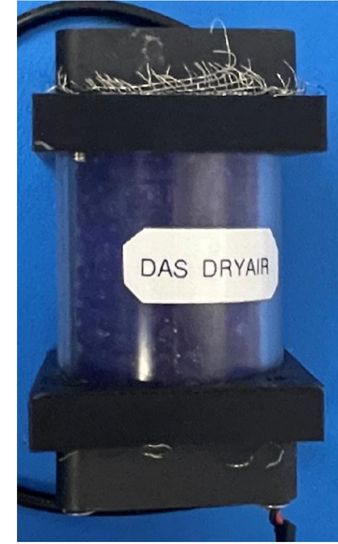
DryAir: Desiccator to reduce the dew point
